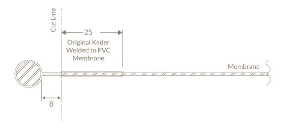
2 AFTER CUTTING OFF OLD KEDER - CLEAN LOCAL AREA PRIOR TO APPLYING NEW KEDER
