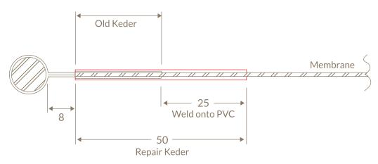
Note: Should a Fabricator prefer to sew on top of the old Keder, it is advisable to High Frequency weld over the sewn area after sewing. This process will allow the PVC from the inside of the Repair Keder to flow and fill any holes created during the sewing process. If sewing we normally recommend using a Twin Needle machine; however this is the choice of the fabricator or repair shop technician.
