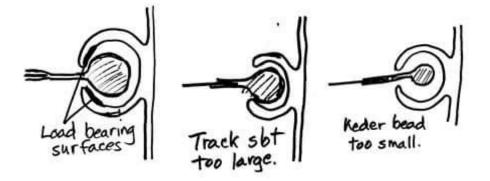
Designers and builders working with tracks have many choices. It is always appropriate to match material and design considerations with known loads and functions. For example, it is common to use 13mm (heavier) attached to tent top fabric but only 11mm attached to side panel fabric in the same size tracks. Overall, the system must retain and support the fabric as intended, withstanding load and stress forces without failure.
