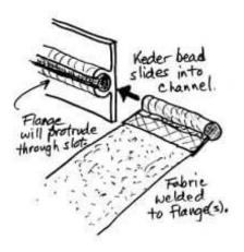
There are many advantages of this system. Fabric structure engineers will note that the connection produces no friction between the sheet and truss, unlike in a structure which employs a cover over a frame. The structures can be strong enough for long-term, semi-permanent installations.
